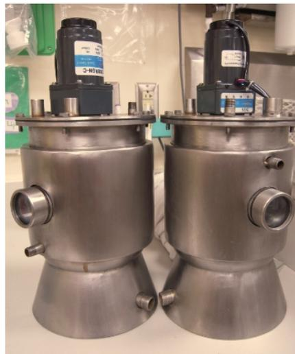
Figure 3. 3-L custom-made bioreactor with pH, O<sub>2</sub>, and temperature probes.
