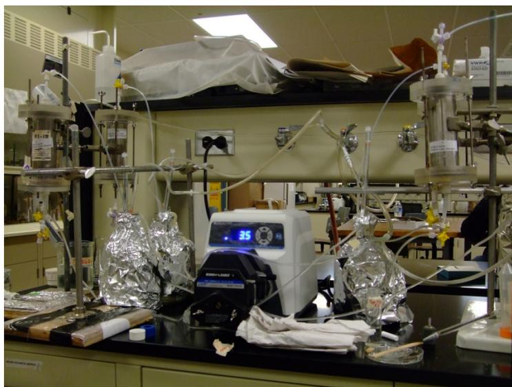
Figure 1. Four columns used for the short-column simulations.
