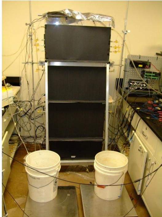
Figure 2. Slab set-up with redox probes, oxygen probes, sampling ports and tensiometers.
