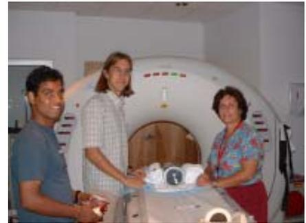
CT scanning of soil core for determination of preferential flow channels.
